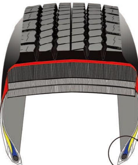
Soft Apex can keep good elasticity of tyre bead, operator comfort and anti-bending performance.
