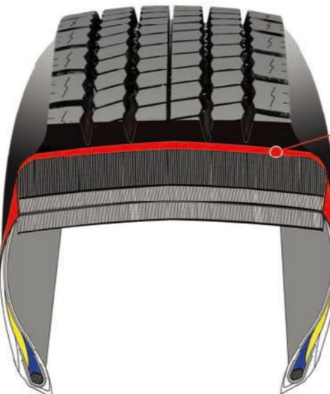
The shoulder wedge in high-stress area should possess excellent fatigue durability and good adhesivity. TRI-NR (Trans-1,4-polyisoprene blend with Natural Rubber) Technology well keeps the tensile strength and tearing strength of tyre compound, while it lowers heating and rolling resistance. This technology can increase adhesivity and decrease hardness at the same time.
